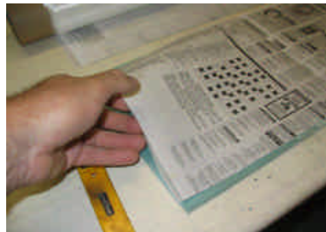
Now take the first skin, with the cloth at 45 degrees and turn it over with the paper holding it in shape and carefully place it on top of the cloth at 90 degrees, lying on the mylar sheet.
