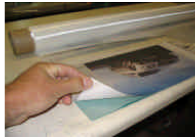
Now, carefully remove the paper without disturbing the fibreglass cloth.
