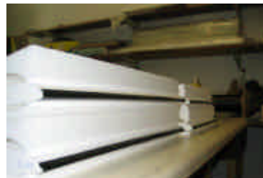
Allow the LE to cure undisturbed overnight
