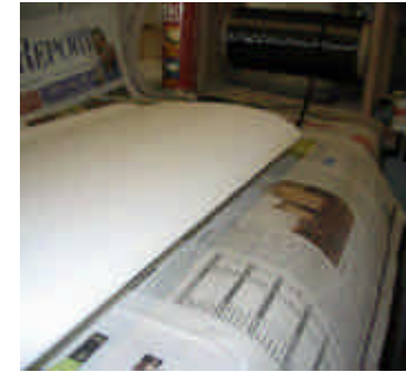
Mark out about 7mm back from the LE on top and bottom. We are going to put 3 tows of 5mm wide carbon onto the LE. One on top one on the front and one underneath.
