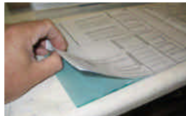
Now take the first skin, with the cloth at 45 degrees and turn it over with the paper holding it in shape and carefully place it on top of the cloth at 90 degrees, lying on the mylar sheet.
