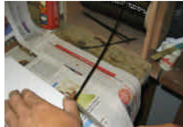
Immediately apply carbon tows to the LE, sticking them down to the wet contact glue
